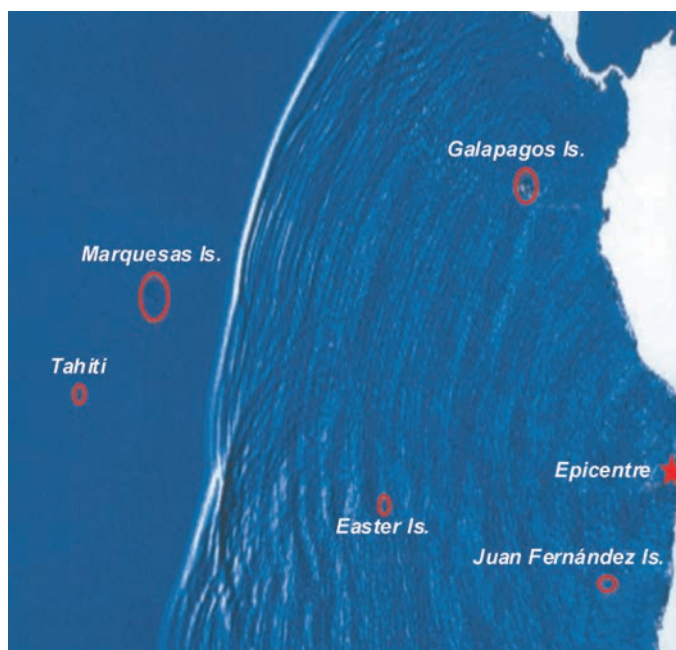
Model of tsunami propagation in the southeast Pacific, nine hours after generation. Source: Antofagasta, Chile (30 July 1995). Courtesy of LDG, France.
